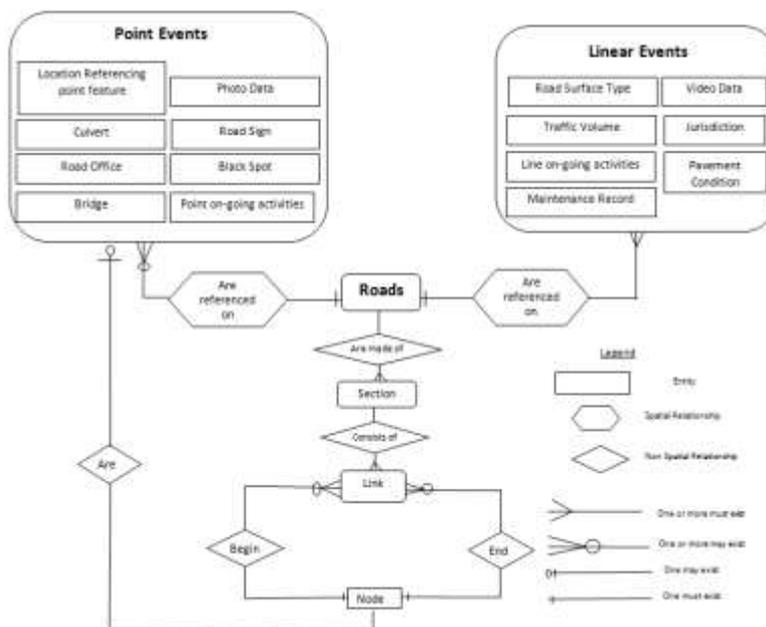
**Figure 1: Conceptual Data Model - Entity Relationship Diagram**
