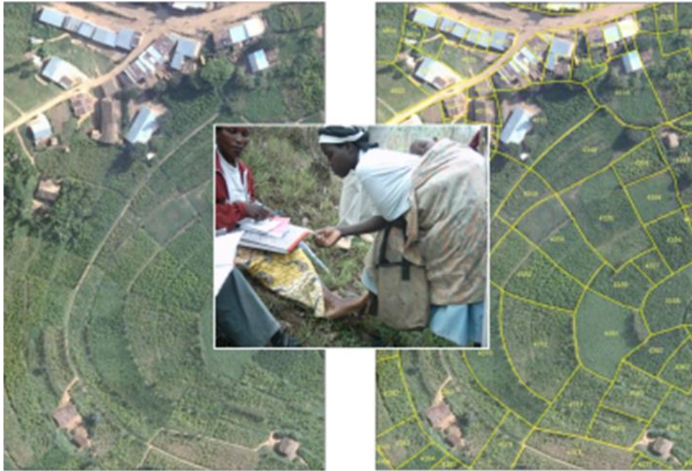
Figure 6: Example from Rwanda showing aerial imagery (left), from which the parcel boundaries are easily identified (right). This is essentially a participatory approach undertaken by locally trained land officers Source: Didier Sagashya, Rwanda
